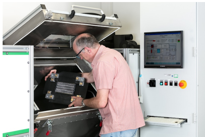
Figure 3: Installation of heating element in the air duct (Lab manager: Hr. Schaeffner)
